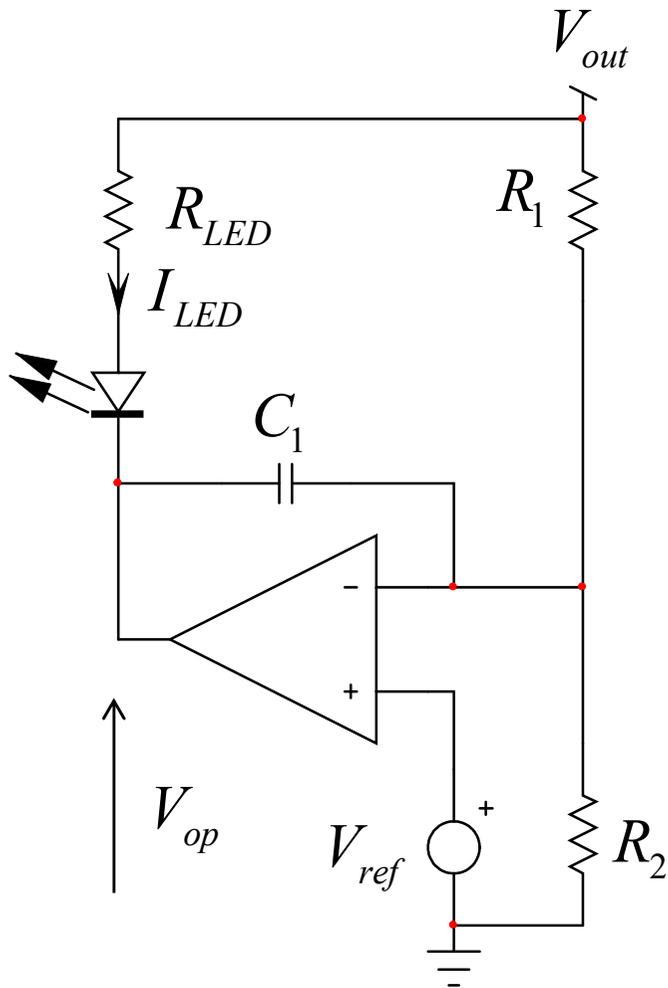
$$I_{LED}(s) = \frac{V_{out}(s) - V_{op}(s)}{R_{LED}}$$
