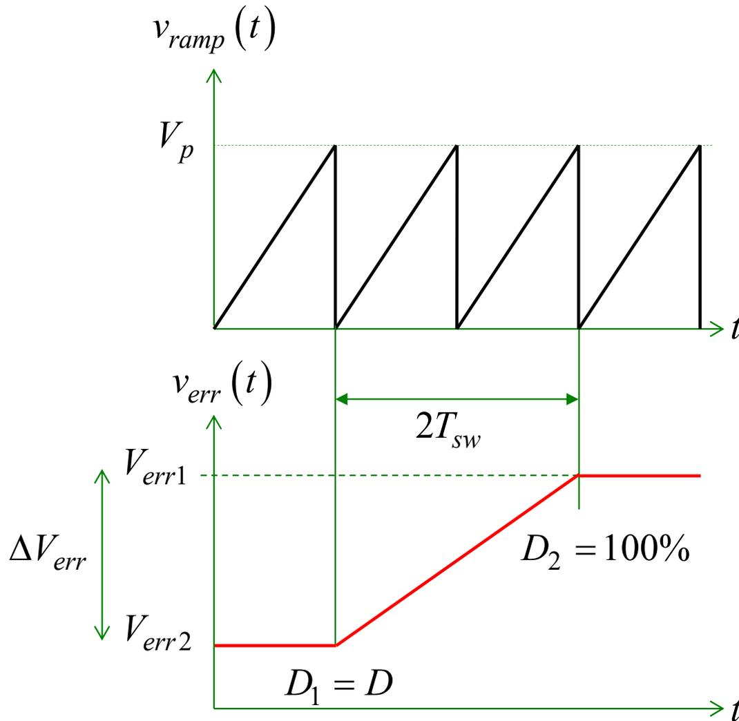
$$SR_2 = \frac{\Delta V_{err}}{2T_{sw}} = \frac{V_{err1} - V_{err2}}{2T_{sw}}$$
