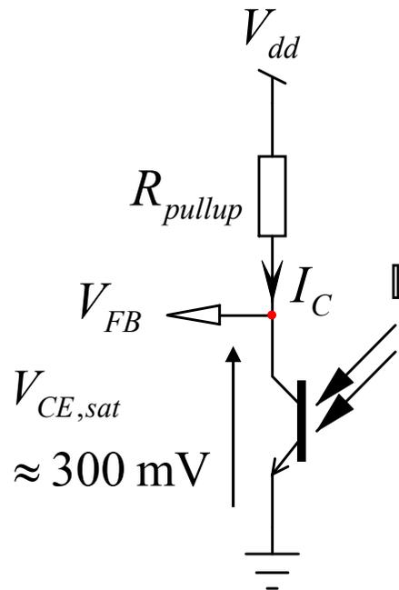
$$I_{C,max} = \frac{V_{cc} - V_{CE,sat}}{R_{pullup}}$$
