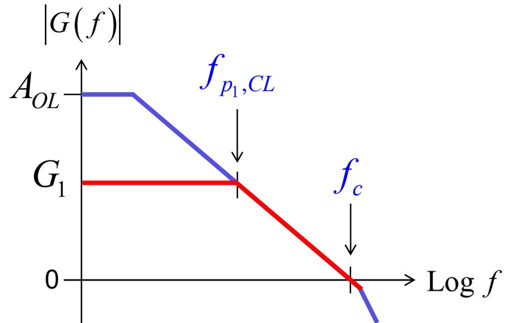
$$S = \frac{\Delta y}{\Delta x} = \frac{-20 \text{ dB}}{\log\left(\frac{10 f_{p1}}{f_{p1}}\right)} = -20 \text{ dB/dec}$$
