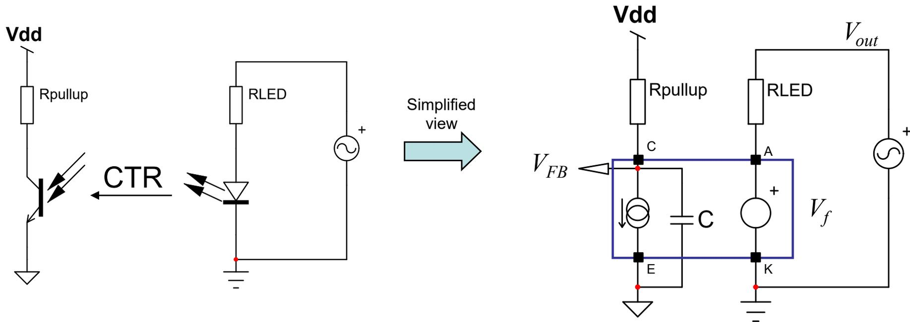
$$\frac{V_{FB}(s)}{V_{out}(s)} = -\frac{R_{pullup} CTR}{R_{LED}} \frac{1}{1 + sR_{pullup} C}$$
