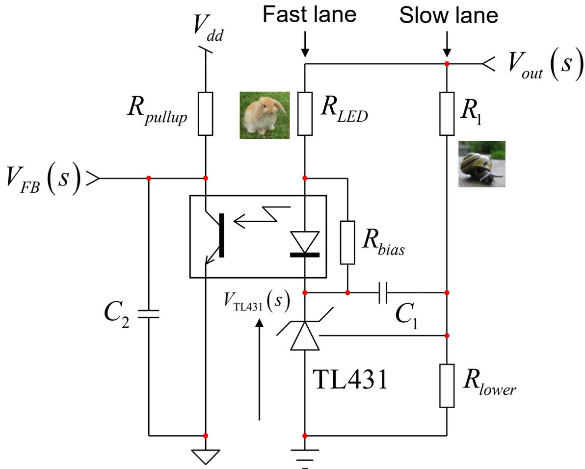
$$I_{LED}(s) = \frac{V_{out}(s) - V_{TL431}(s)}{R_{LED}}$$
