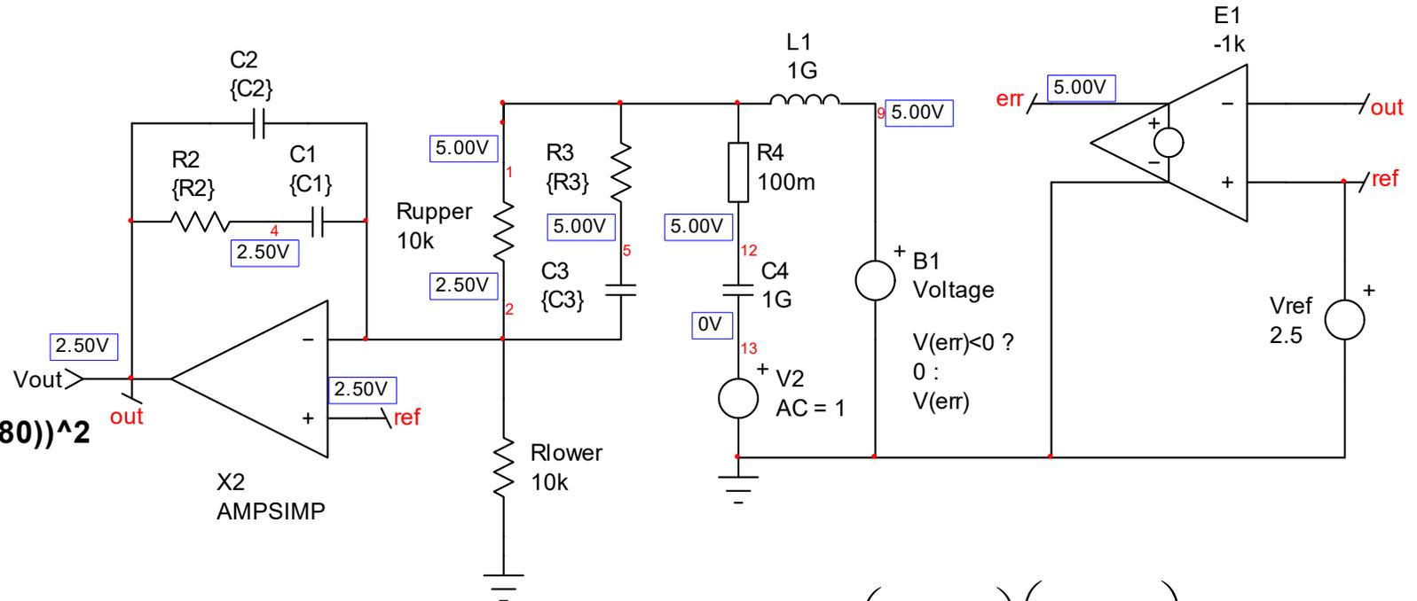
$$G(s) = -G_0 \frac{\left(1 + \frac{s}{z_1}\right) \left(1 + \frac{s}{s_{z_2}}\right)}{\left(1 + \frac{s}{s_{p_1}}\right) \left(1 + \frac{s}{s_{p_2}}\right)}$$
