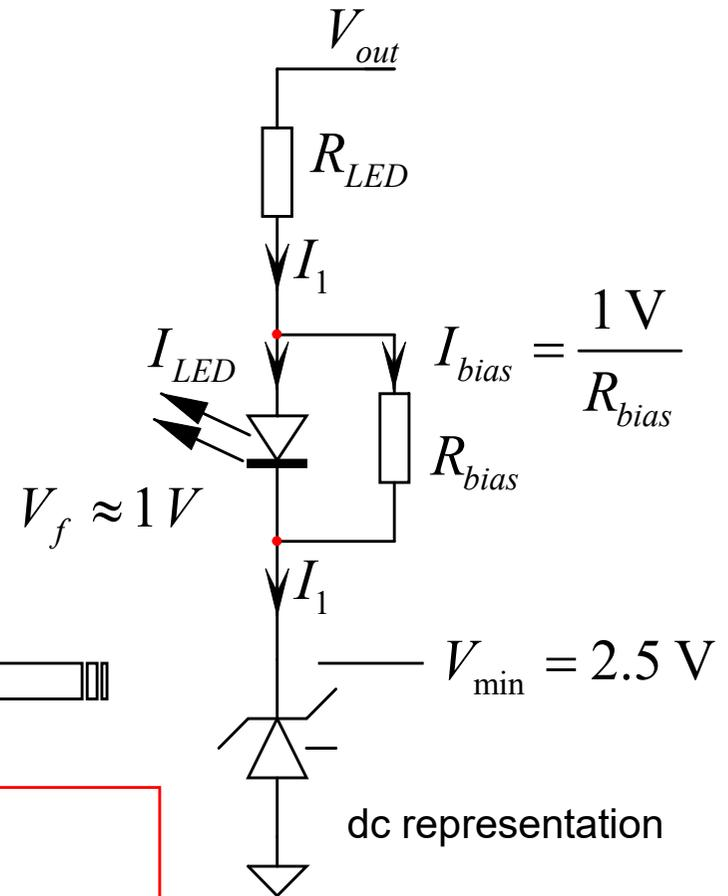
$$R_{LED,max} = \frac{V_{out} - V_f - V_{TL431,min}}{V_{dd} - V_{CE,sat} + I_{bias} CTR_{min}} R_{pullup} CTR_{min}$$
