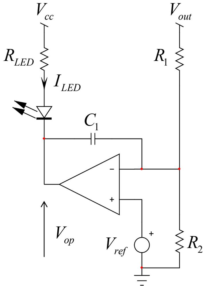
$$I_{LED}(s) = \frac{\cancel{V_{cc}} - V_{op}(s)}{R_{LED}} = -\frac{V_{op}(s)}{R_{LED}}$$
